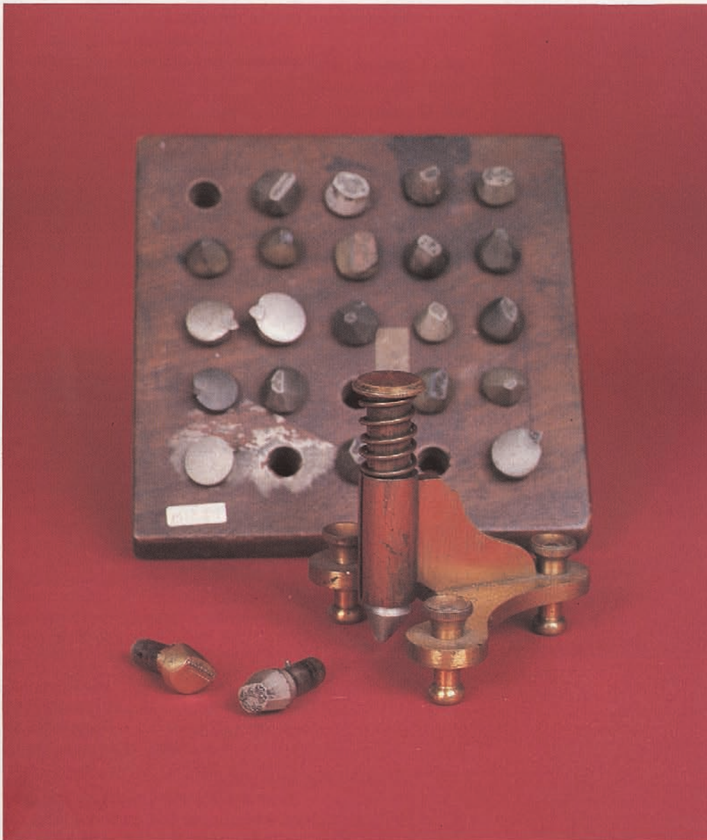
Engraver's spring-punch with a selection of tree and vegetation stamps.
