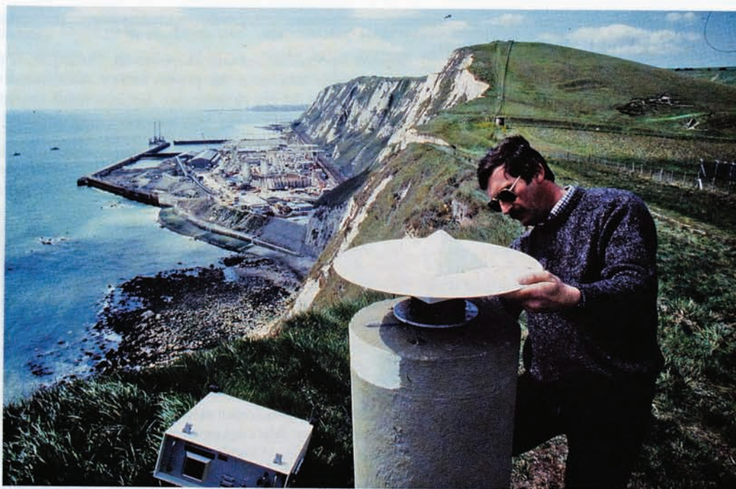
Global Positioning System equipment in use near the Channel Tunnel workings.
