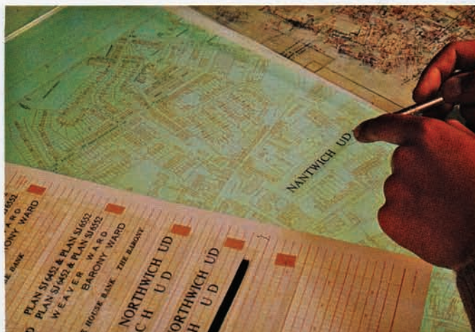
Application of lettering to a large-scale map.
