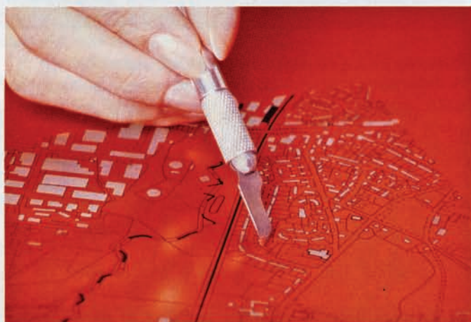
Peeling out sections of a plastic sheet to expose building detail on the scribed underlay.
