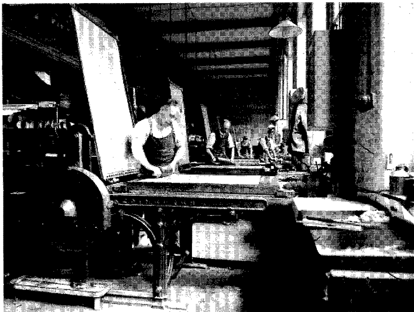
Proving section in the 1920s. Paper was placed on the hand-inked litho-stone and the 'Tinpan' cover lowered over it. The whole bed was rolled through a compression roller to transfer the image onto the paper and provide a proof copy.
